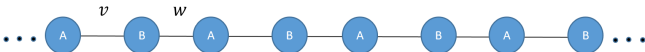
FIG. 3: 1D chain in the SSH model. A sites form a Bravais lattice with parameter a . We are interested in the bulk properties, so we will consider periodic boundary conditions.
