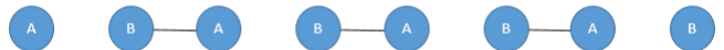
FIG. 1: Schematic representation of a finite chain in the SSH model. If we restrict the electron hopping allowing only B to A movement, 2 edge sites will be left isolated: zero-energy edge states localized at the A and B limits of the chain will appear.
