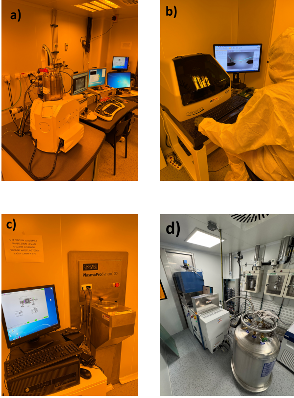
Figure 2: USAL-Nanolab Clean Room: a) FE-SEM and Raith nanolithography system. b) Profilometer system. c) Software control and load-lock chamber for PlasmaPro 100 Estrelas ICP-RIE. d) Main room PlasmaPro 100 Estrelas ICP-RIE.
