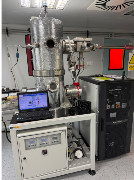
Figure 3: USAL-Nanolab Clean Room: E-beam evaporator.
